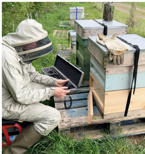
Using hive endoscopy in a National brood chamber
